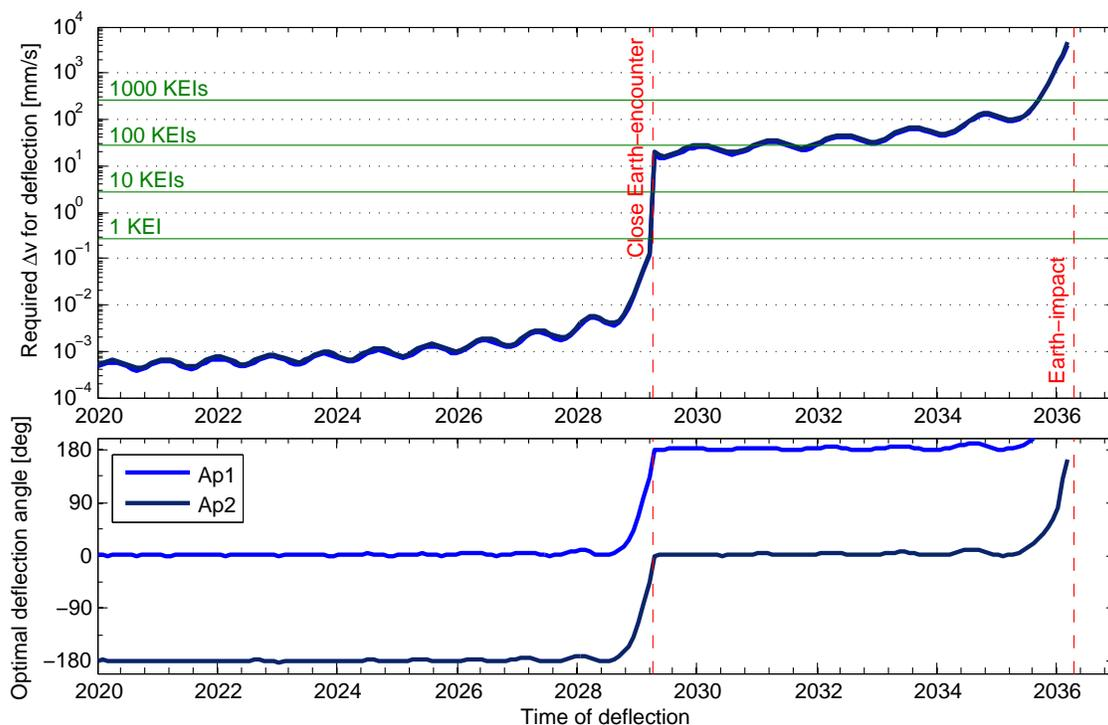
Figure 7. Required velocity change and optimal deflection angle for Ap1 and Ap2
