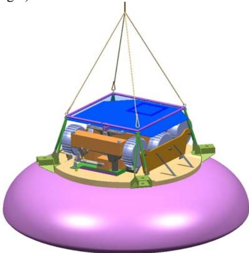
Fig.7: View of ExoMars rover on descent module with inflated 'deadbeat' airbag and parachute attachment (Astrium UK concept).
