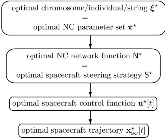
Figure 3: Transformation of the optimal chromosome into the optimal trajectory
