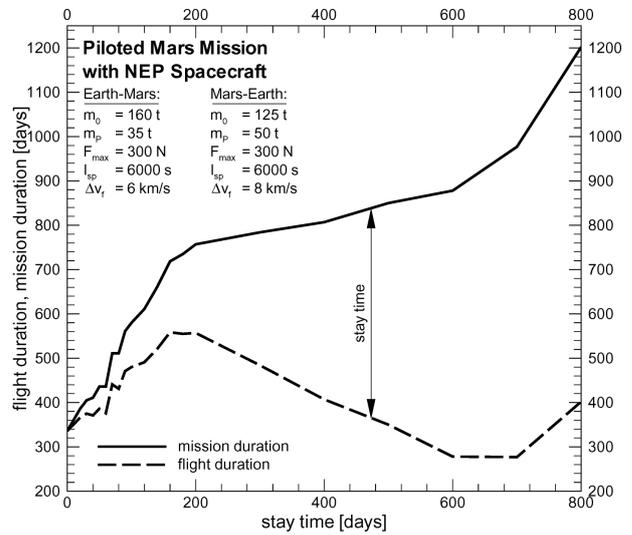
Figure 13: Mission duration against stay time at Mars ( $r_{min} = 0.7$  AU)
