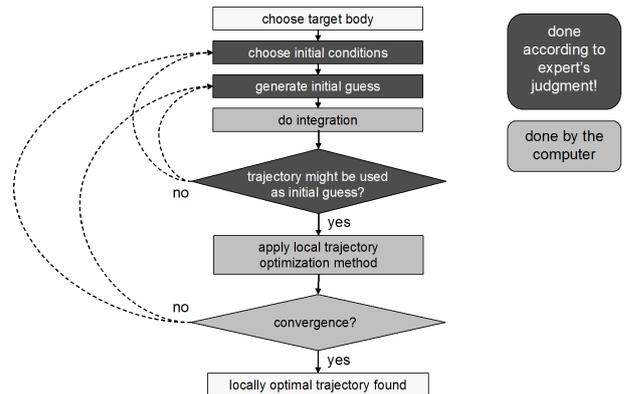
Figure 1: Low-thrust trajectory optimization using a local trajectory optimization method
