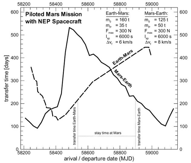
Figure 12: Transfer times against arrival/departure date at Mars ( $r_{min} = 0.7$  AU)
