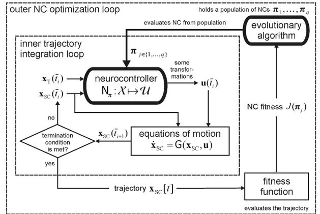
Figure 4: Low-thrust trajectory optimization using evolutionary neurocontrol
