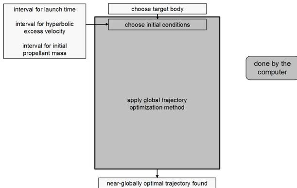
Figure 2: Low-thrust trajectory optimization using a smart global trajectory optimization method
