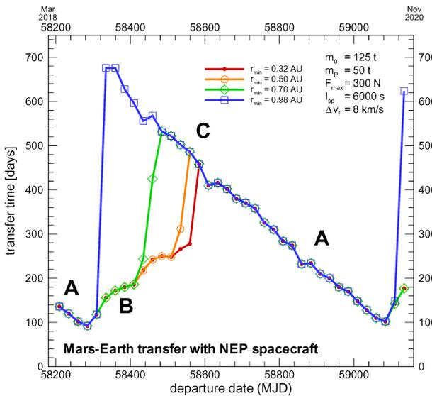
Figure 11: Transfer time for Earth return in dependency of the departure date at Mars and the minimum tolerable solar distance  $r_{min}$
