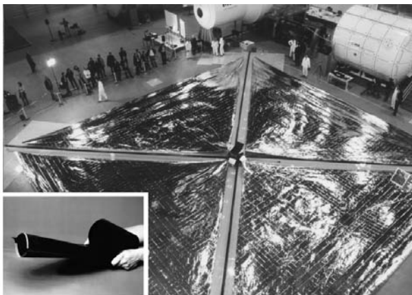
Figure 2: Deployed (20\text{ m})^2 solar sail and CFRP boom at DLR
