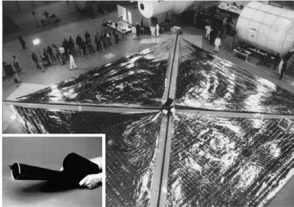
Figure 3: Deployed (20 \text{ m})^2 solar sail and CFRP boom at DLR
