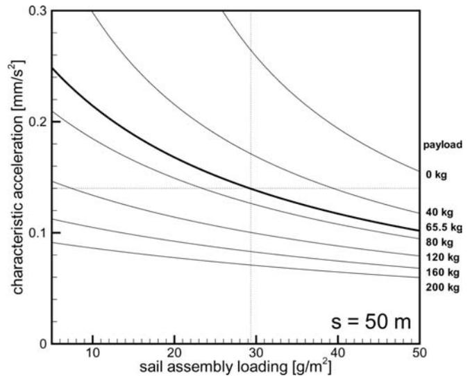
Figure 9: The characteristic acceleration  $a_c$  as a function of  $\sigma_s$  and  $m_p$  for  $s = 50 \text{ m}$
