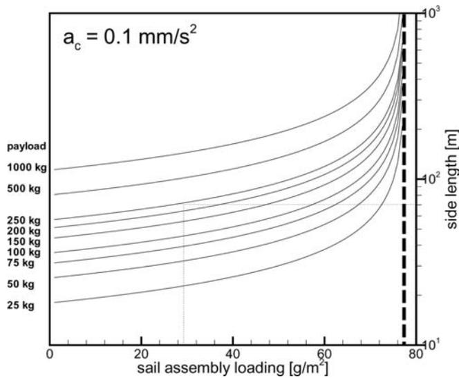
Figure 12: The side length  $s$  of the solar sail that is required to achieve a characteristic acceleration of  $0.10 \text{ mm/s}^2$  as a function of  $\sigma_s$  and  $m_p$
