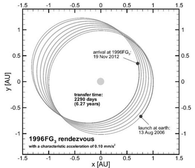
Figure 10: 1996FG<sub>3</sub> rendezvous trajectory for  $a_c = 0.10 \text{ mm/s}^2$
