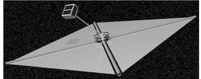
Figure 6: DLR ENEAS solar sailcraft with deployed control mast (artist's view)
