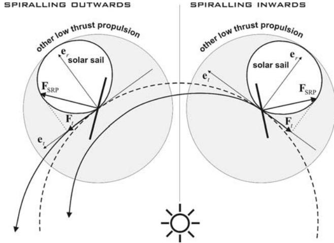
Figure 3: Spiralling inwards and outwards
