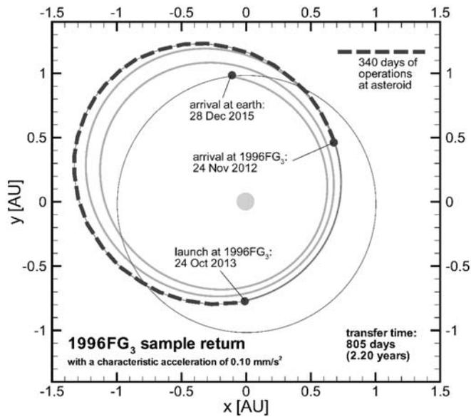
Figure 11: 1996FG<sub>3</sub> sample return trajectory for  $a_c = 0.10 \text{ mm/s}^2$
