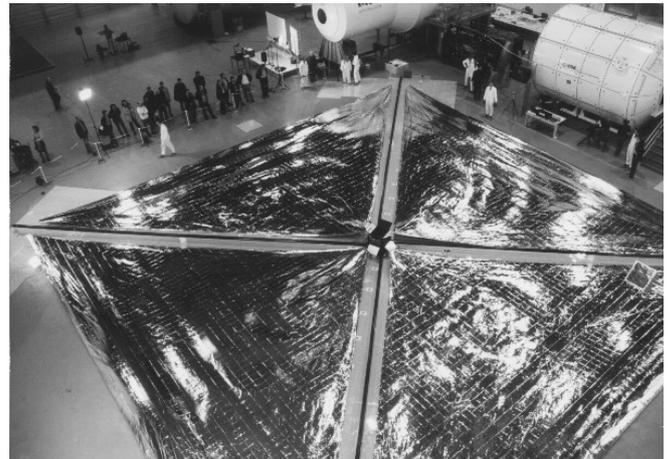
Figure 4: Fully deployed  $20 \text{ m} \times 20 \text{ m}$  solar sail at DLR
