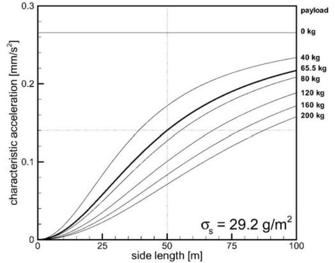
Figure 8: The characteristic acceleration  $a_c$  as a function of  $s$  and  $m_p$  for  $\sigma_s = 29.2 \text{ g/m}^2$
