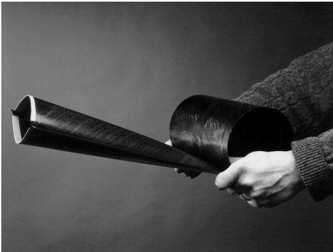
Figure 5: DLR deployable CFRP boom
